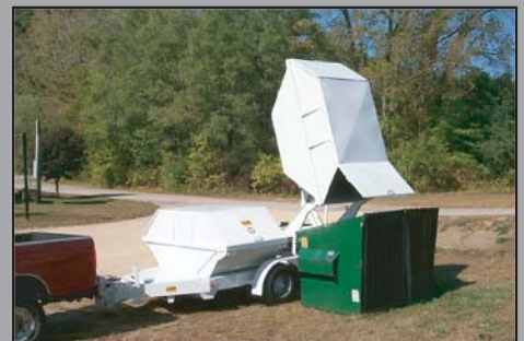
Side Dump containers dump independently.
