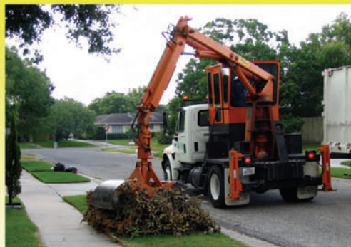
Saves time because outriggers not needed for most loads
