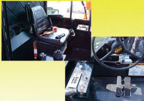
Climate controlled operator cab includes all driving controls plus twin joysticks for loader operation
