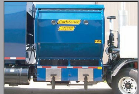
Trough Loader containers can have up to two cart tipper per trough.
