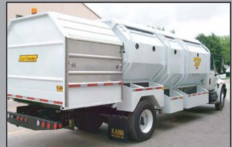
A variety of container and compactor options allow for efficient collection of numerous commodities and eliminates cross contamination.
