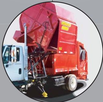
Trough Loader ® Container/Compactor Can Be Installed In Front Of Rear Loaders For Multi-Commodity Collection
