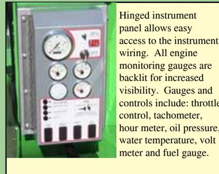
Hinged instrument panel allows easy access to the instrument wiring. All engine monitoring gauges are backlit for increased visibility. Gauges and controls include: throttle control, tachometer, hour meter, oil pressure, water temperature, volt meter and fuel gauge.
