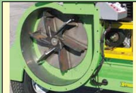
Bolt-in liners are located in the blower housing to reduce housing wear. The liners are easy to change and helps save money and downtime.
