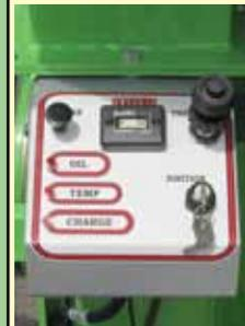
Engine controls and gauges include: tachometer, hour meter, throttle, choke and keyed ignition switch. Indicator lights for low oil pressure, high engine temperature and battery charging are included.
