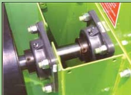
The impeller turns on two heavy-duty, 1.5" diameter flange bearings.
