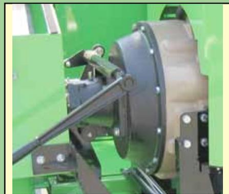
The PTO/Clutch is a heavy duty 13" automotive style assembly.
