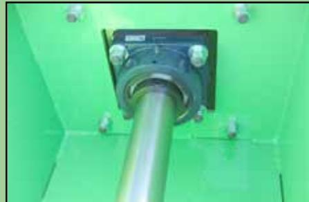
The drive bearings assembly consists of two heavy duty four bolt flange bearings with double row, precision spherical roller bearings.
